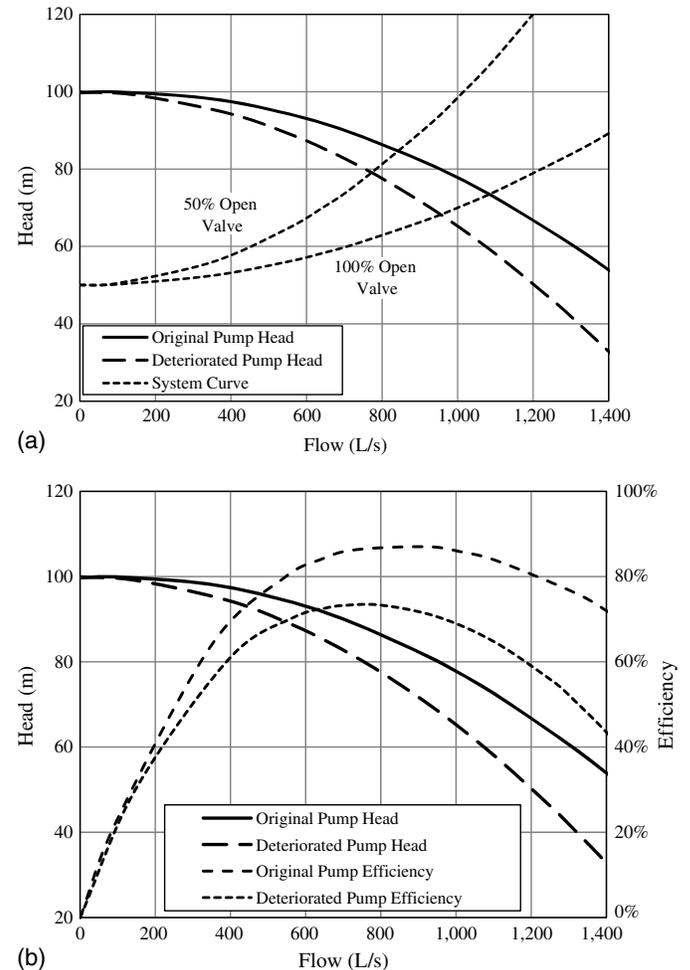
**Fig. 3.** Original and deteriorated pump curves and system curve: (a) pump performance and system curves; (b) pump performance and efficiency curves
