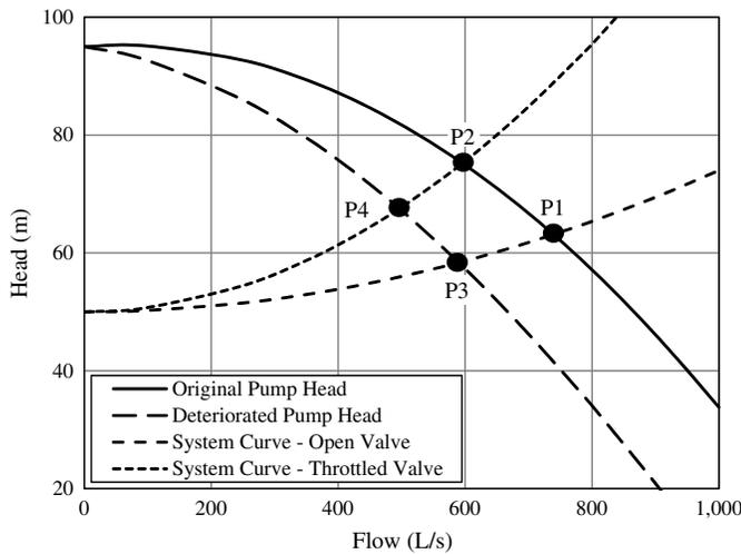
**Fig. 2.** Example pump and system curves showing the range of potential operating points
