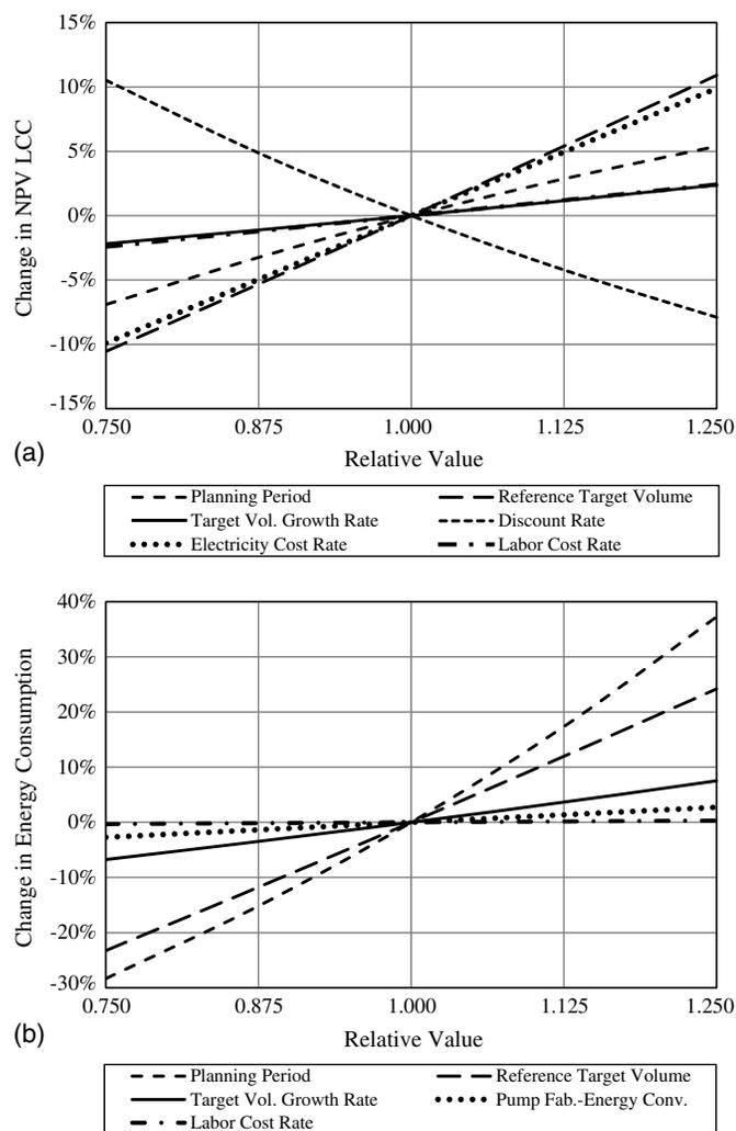
**Fig. 6.** Sensitivity plots for select parameters: (a) NPV LCC; (b) energy consumption
