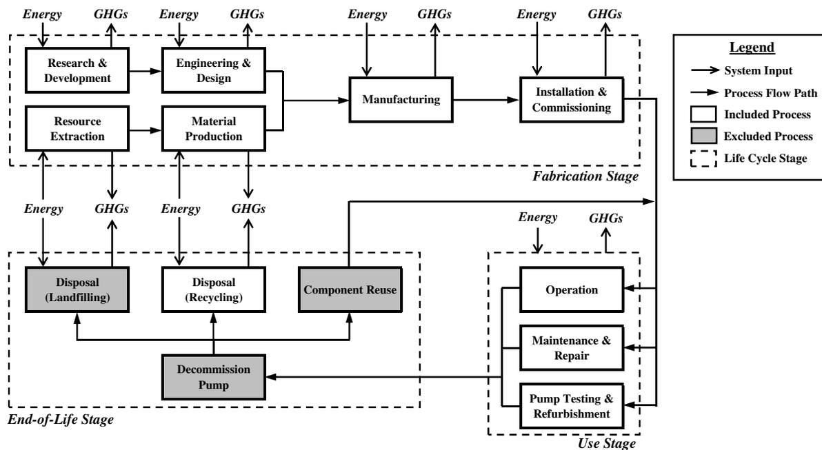
Fig. 1. Lifecycle stages, processes, and system boundaries of a WDS pump
