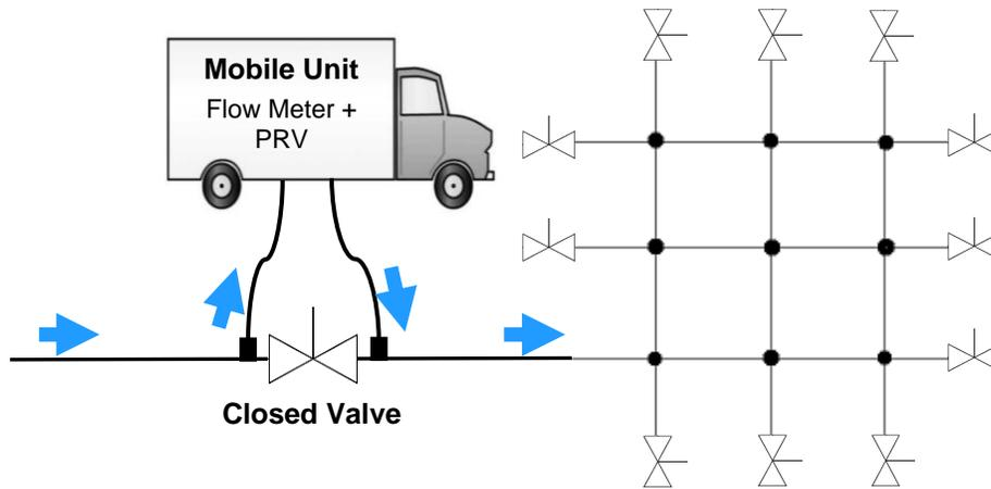
Figure 3: Mobile testing unit concept
