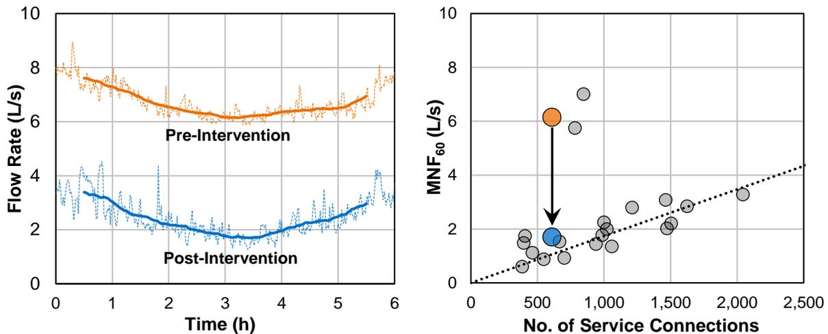
Figure 6: Pre- and post-intervention flow profiles (left) and benchmarking results (right)
