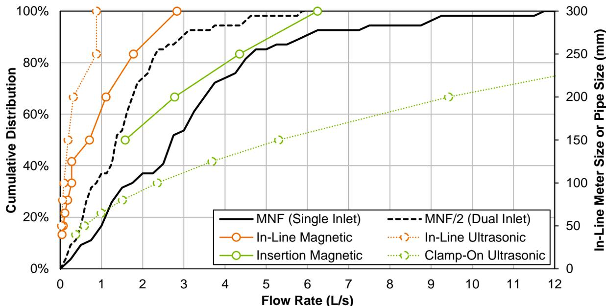
Figure 2: Distribution of DMA sizes in representative city relative to flow metering technology capabilities
