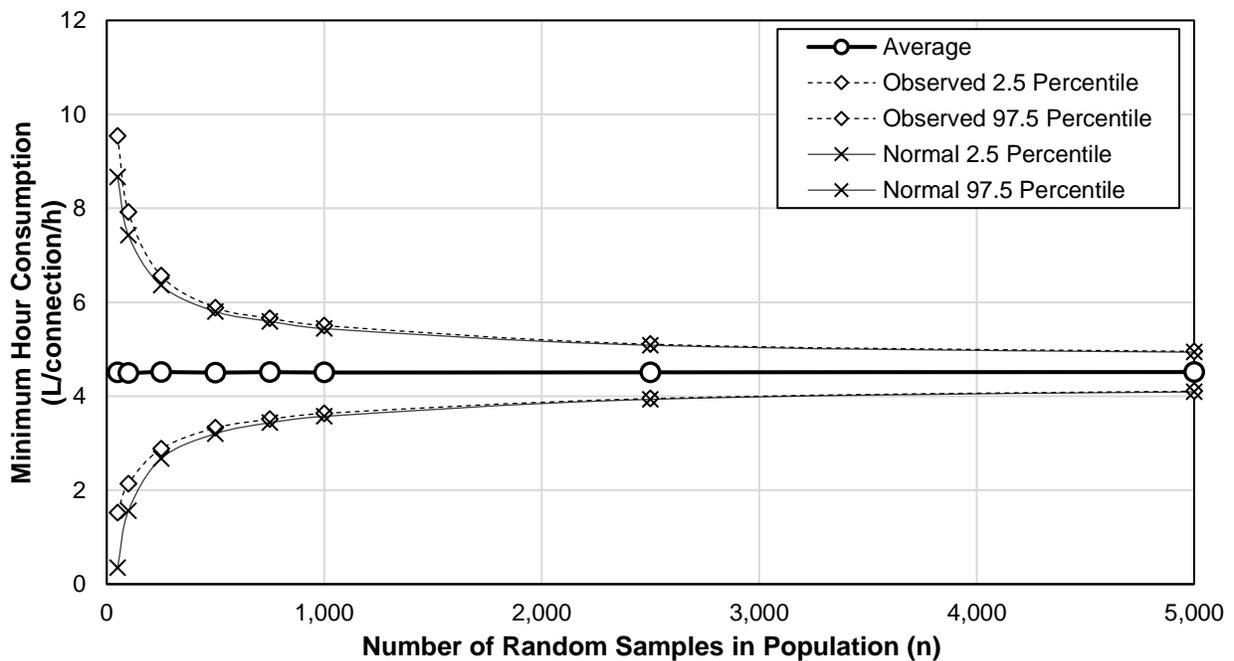
Figure 8: AMI bootstrap analysis results illustrating the relationship between variability and sample size
