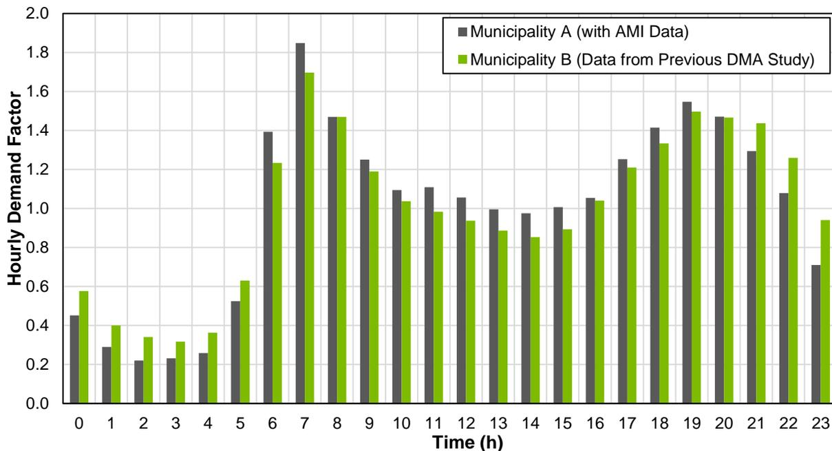
Figure 7: Diurnal AMI consumption and flow profiles
