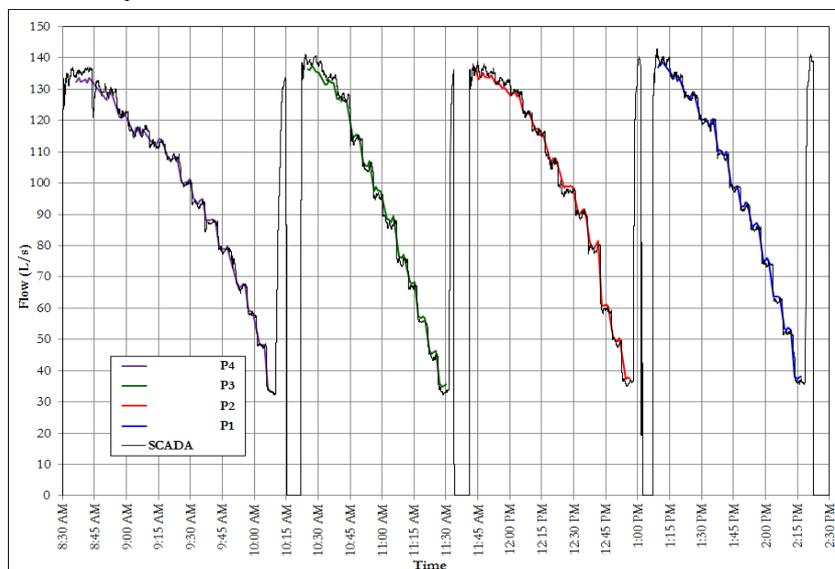
*Figure 4. Example of a Favourable Comparison between Flow Rates using the Thermodynamic Pump Testing Method and Pump Station Flow Meter*
