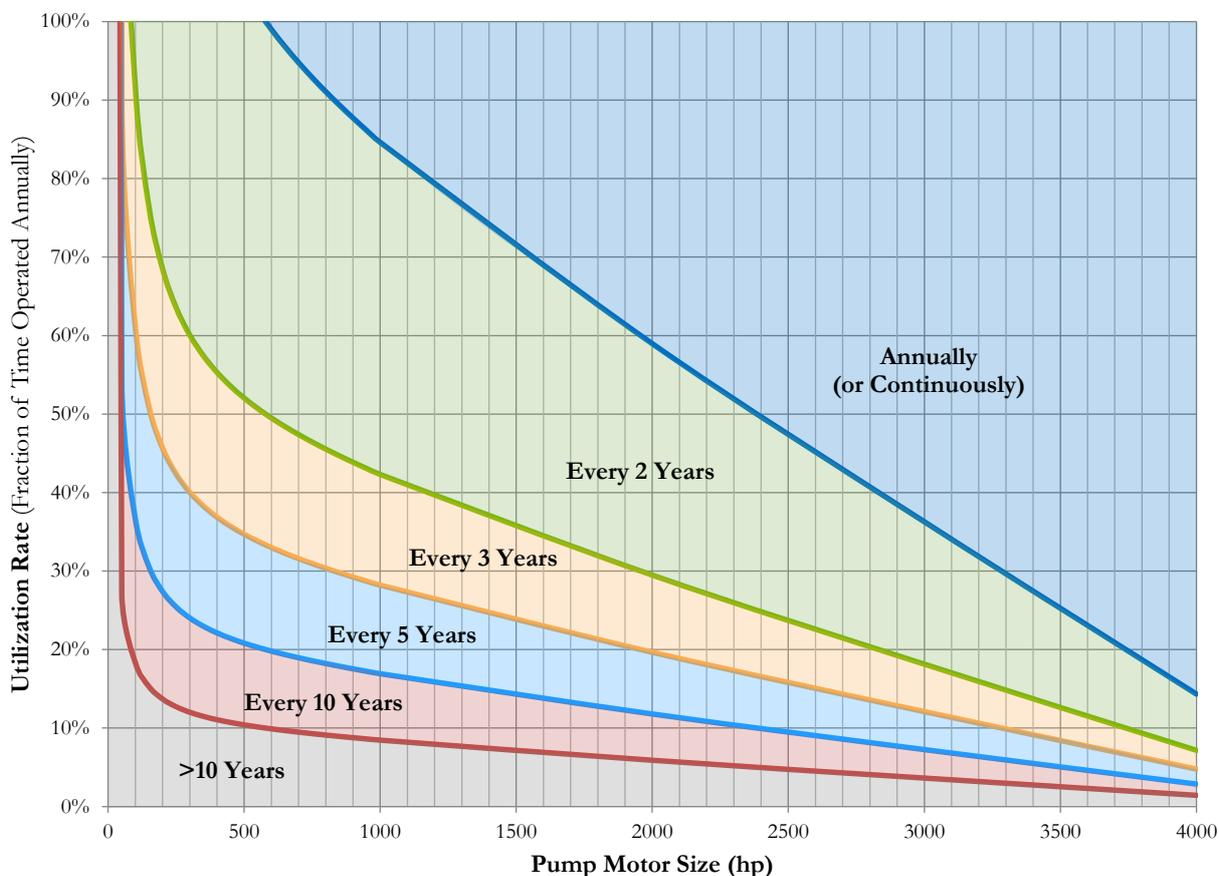
Figure 2. Guideline for Pump Testing Frequency [1]
