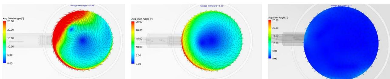
*Figure 6. CFD Modelling of Hydrodynamic Flow Regime at Flow Meter Location for Progressive Re-Design Iterations*
