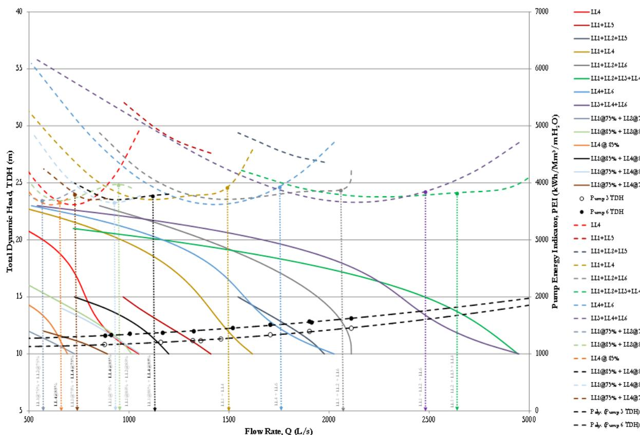
Figure 3. Using the Pump Energy Indicator (PEI) Metric to Optimize Pump Selection
