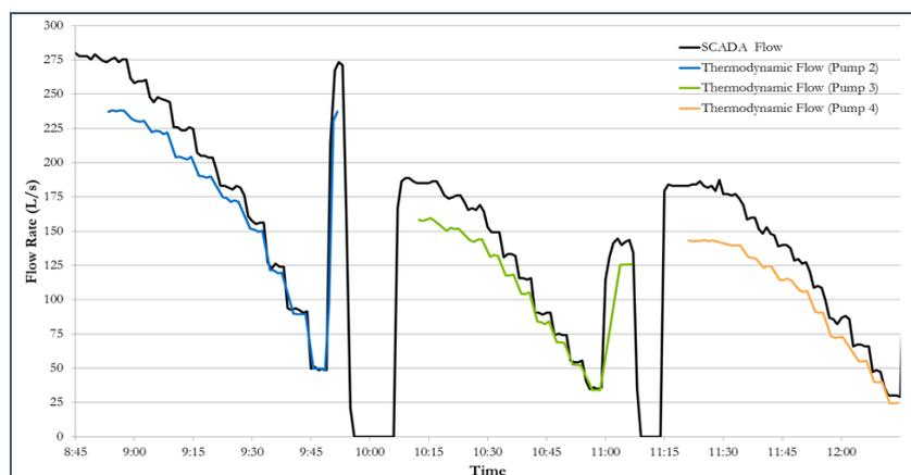
*Figure 5. Example of Pump Station Flow Meter Inaccuracy as identified using the Thermodynamic Pump Testing Method*
