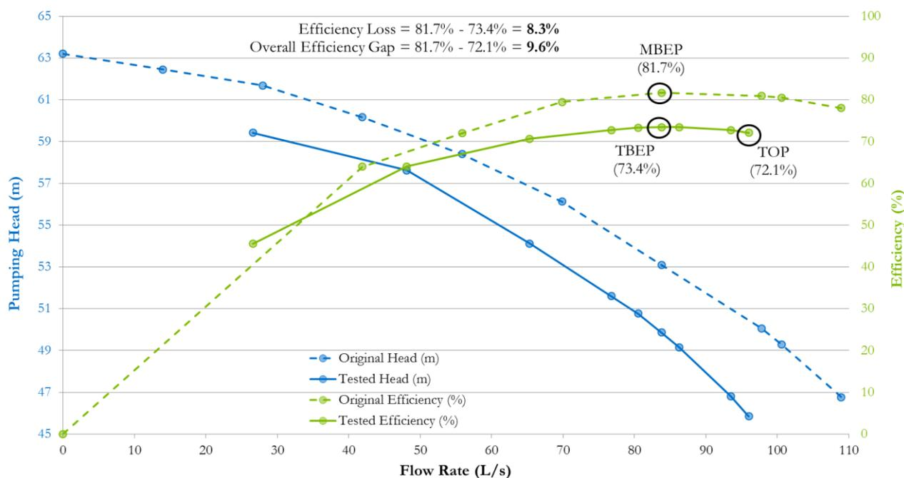
Figure 1. Example of Actual Pump Performance Characteristics as Measured in the Field Compared to Original Manufactured Condition [1]
