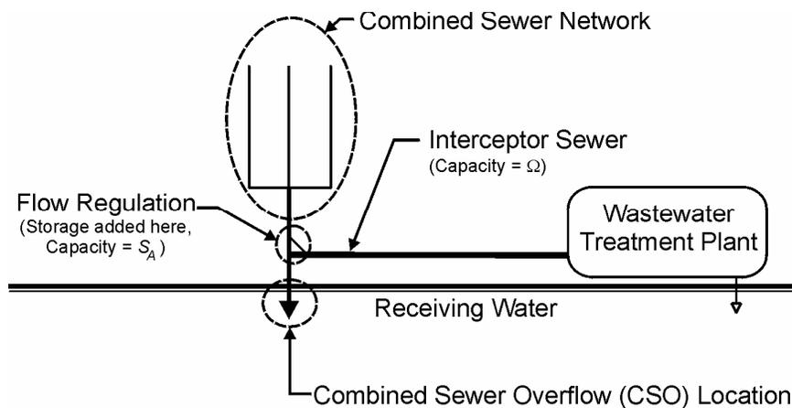
**Figure 1.** Schematic representation of combined sewer network.
