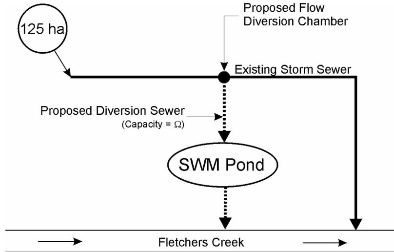
**Figure 6.** Schematic representation of Alternative 3.
