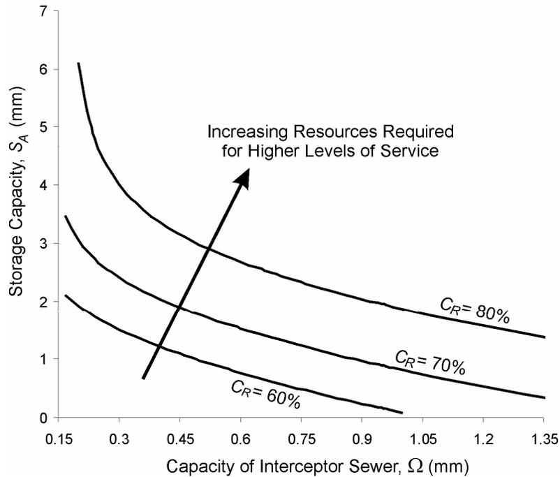
**Figure 3.** Isoquants of runoff control.
