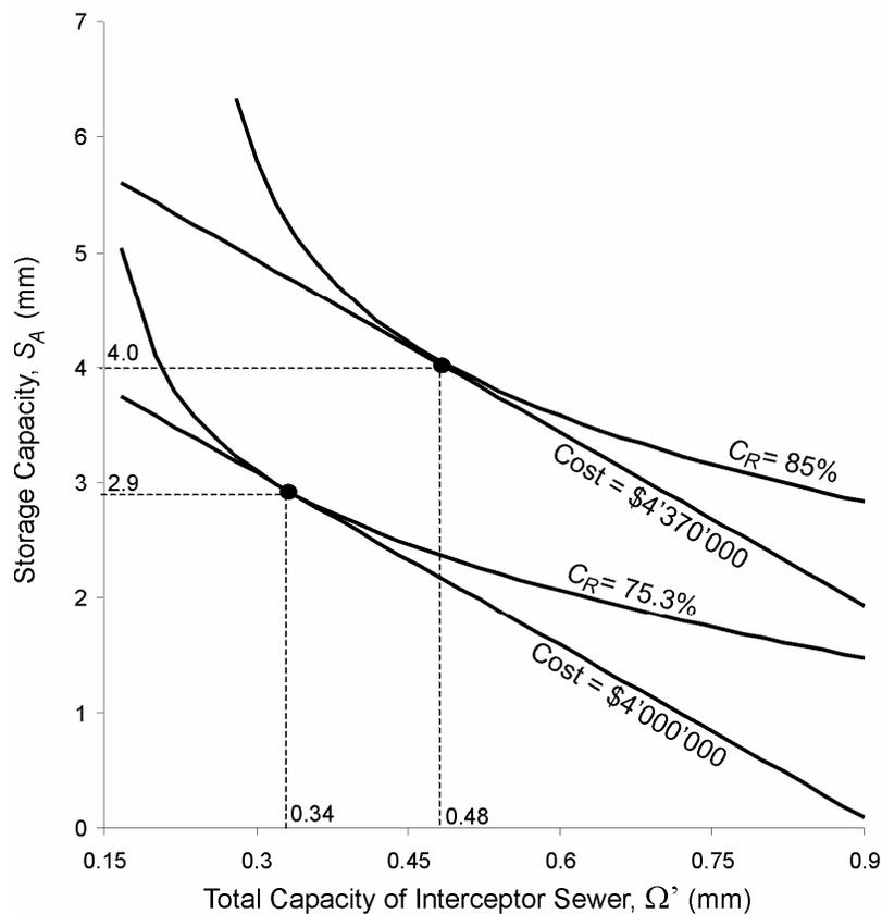
**Figure 4.** Selection of optimal design variables.
